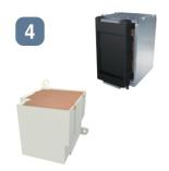
This is the device that automatically trips the breaker when the circuit voltage drops below the nominal voltage, and comprises UVT coil and UVT controller. There are 3 kinds of tripping time, INST, 0.5s and 3.0s.
